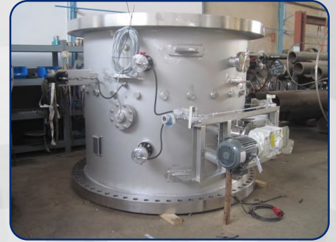
External side with motor and head loss sensor
