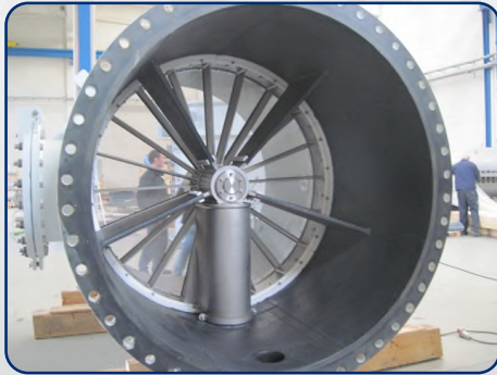
Upstream side with suction scoop
