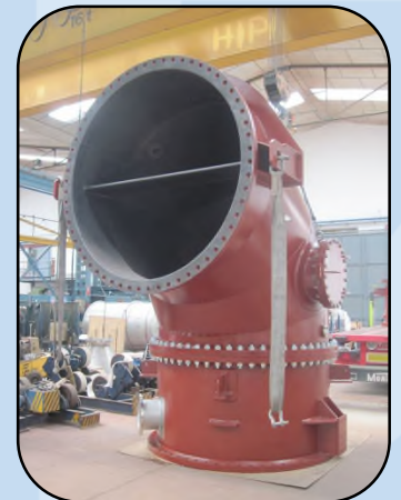
Big elbow filter Dia.=2.1m
