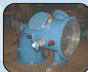
Small elbow filter Dia.=0.6m
