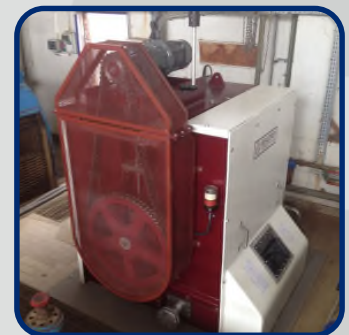
Indirect transmission with chain
